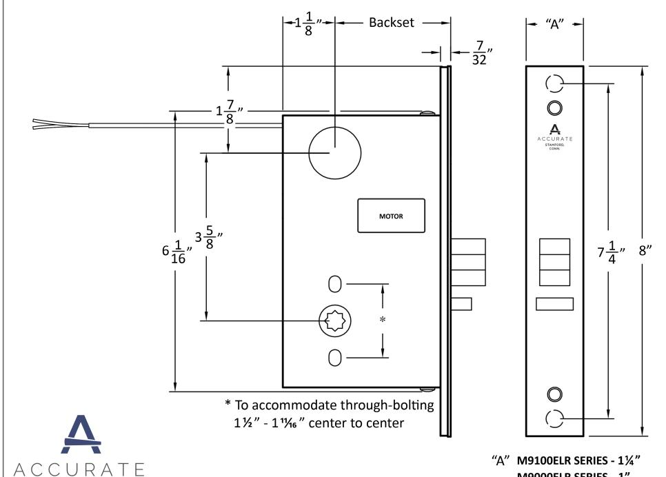
M9100ELR - Motor Drive Electrified **Latch Retraction Mortise Locks**
